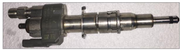
Injector removed from cylinder head
