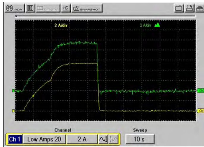
Figure C-7 Sample Noise Filter—two low amp scope probes
