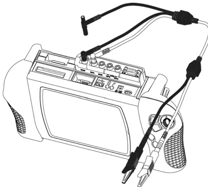
Figure 2-1 Sample yellow lead connection
