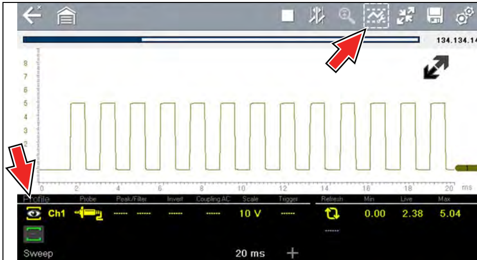
Figure 10-11 Control Panel - Channel Controls
