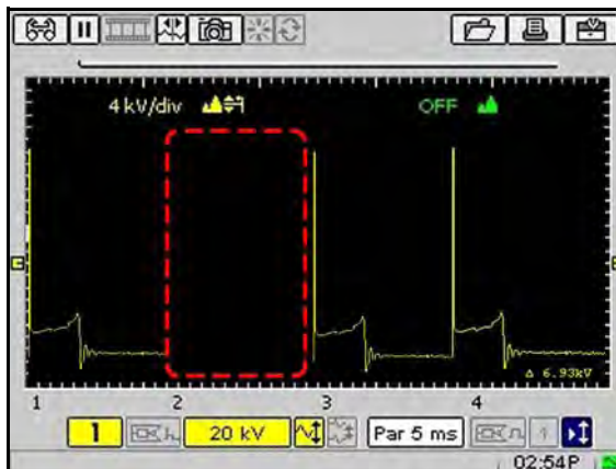
Figure 7-10 Sample missing cylinder detection
