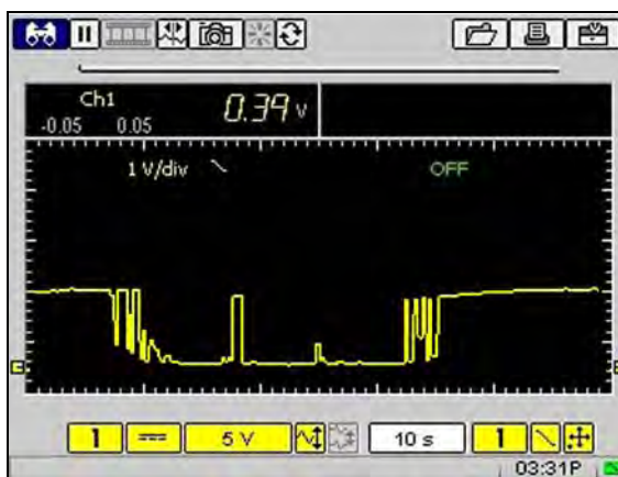
Figure B-6 Sample Faster Sweep—TPS Glitch captured
