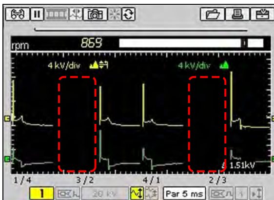
Figure D-9 Sample 6/3 coil not firing and not detected
