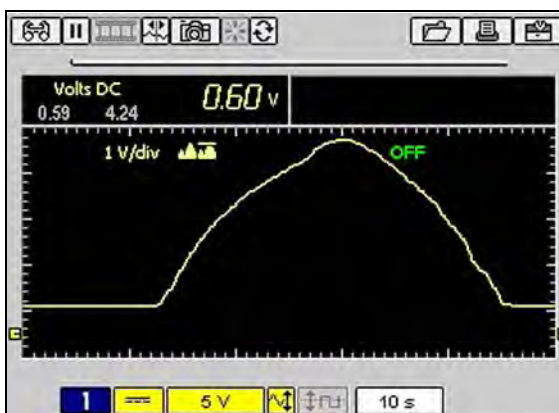
Figure C-4 Sample of Noise Filter on—TPS Sweep (KOEO)
