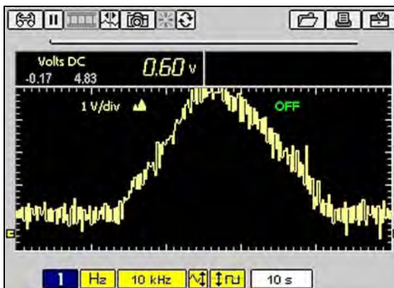
Figure C-3 Sample Noise Filter off—TPS Sweep (KOEO)
