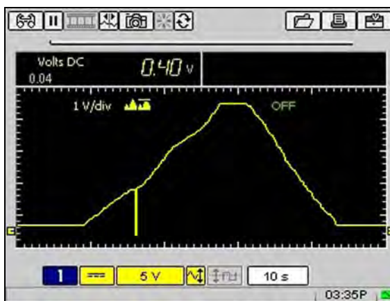
Figure B-7 Sample 10 Second Sweep—TPS Glitch captured
