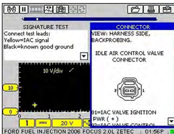
Figure 5-11 Sample connection instructions
