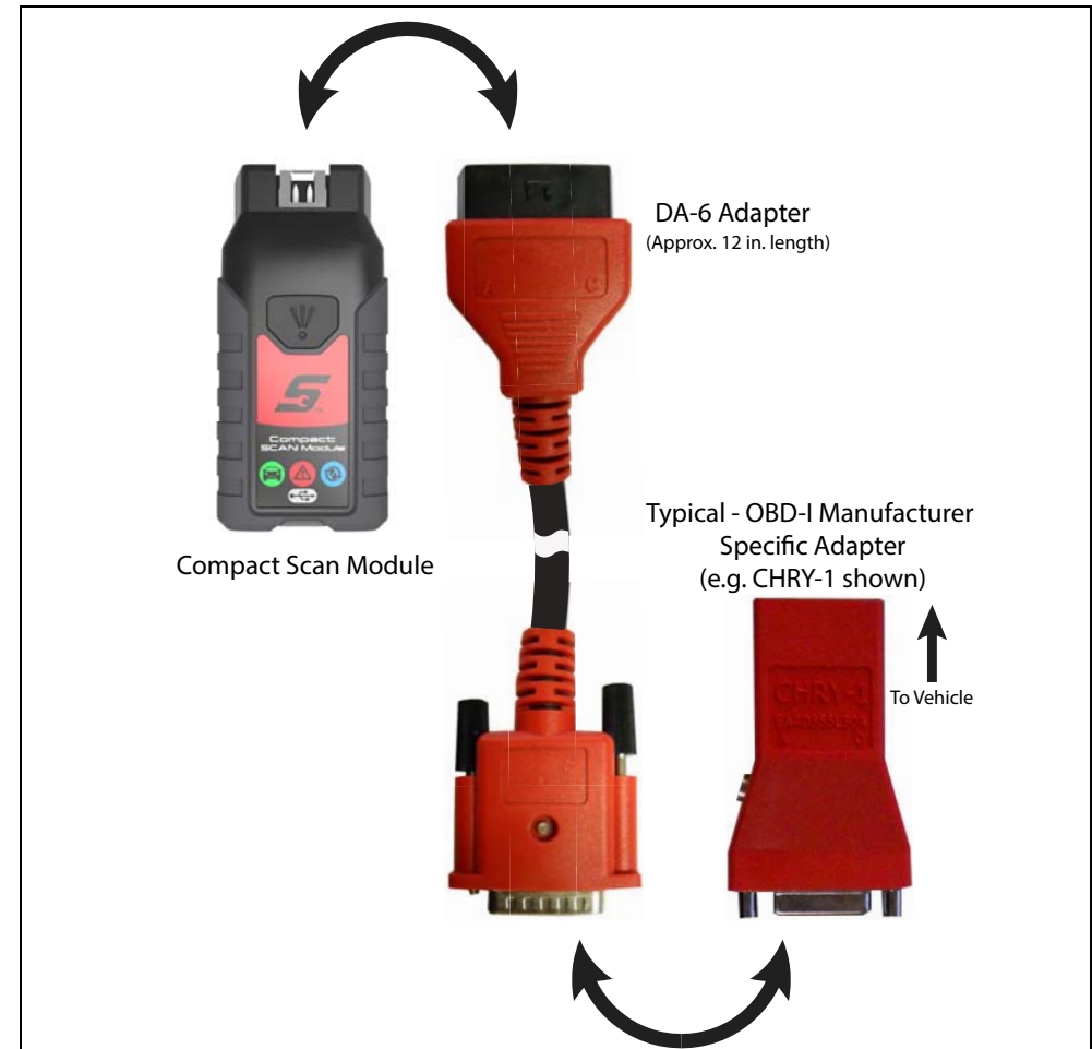
Figure 3-3 OBD-I DA-6 Connection Example
