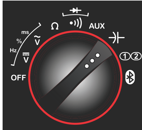
Figure 5-10 Sample capacitance selected
